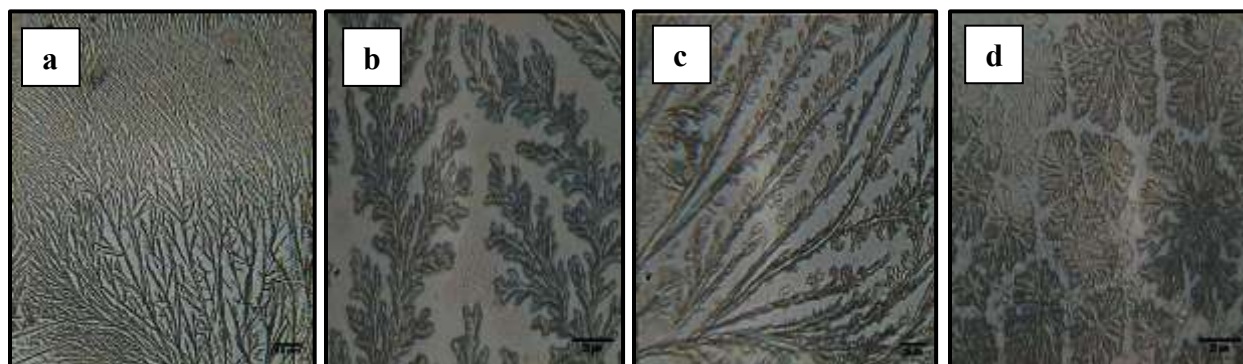
Figure 7 Effect of pH in the self-assembled structure of Sodium Carboxymethyl cellulose (a) pH=3.5, (b) pH=4.0, (c) pH=4.5, (d) pH=5.3.
