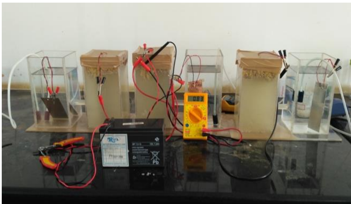
Fig- 1: The experimental setup of Double-Chamber MFC
