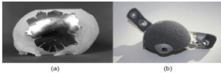
Fig. 5. (a) Stereolithographic resin model of a full skull with a custom Ti plate in place; (b) hip implant fabricated by SLM Solutions in Germany [14].
