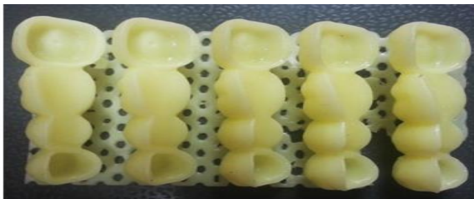
Fig 19- Polymer temporary bridges,produced by stereolithography
