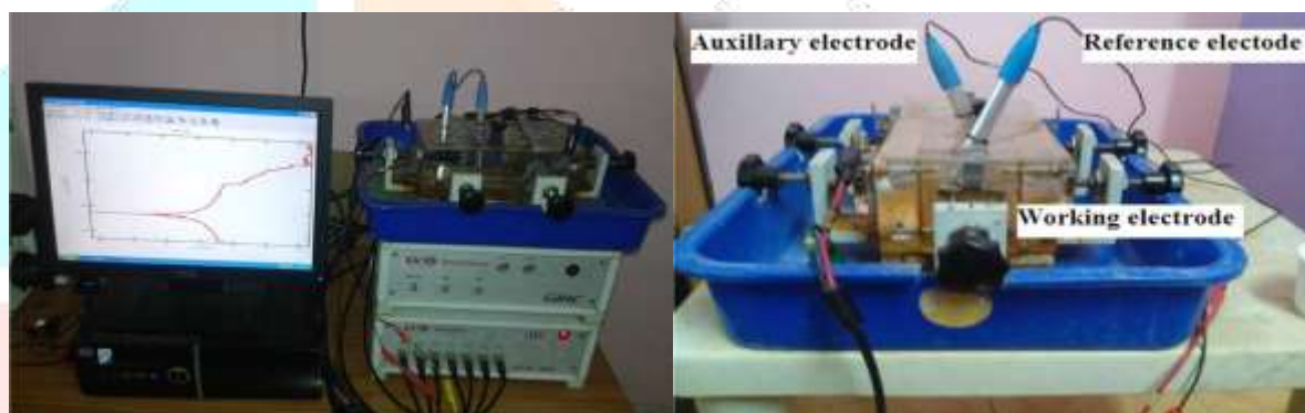
Fig. 1 Basic Electrochemical System for corrosion testing (Gill AC)
