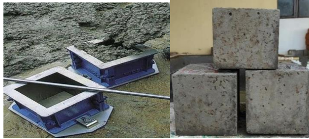
Fig. 1 Before and After Casting of Concrete
