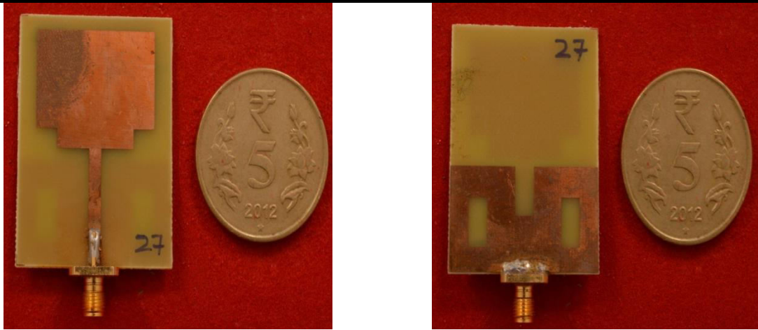
Fig. 2 Photographs of the top and bottom view of fabricated SDSSSPGWimaxNBMSA
