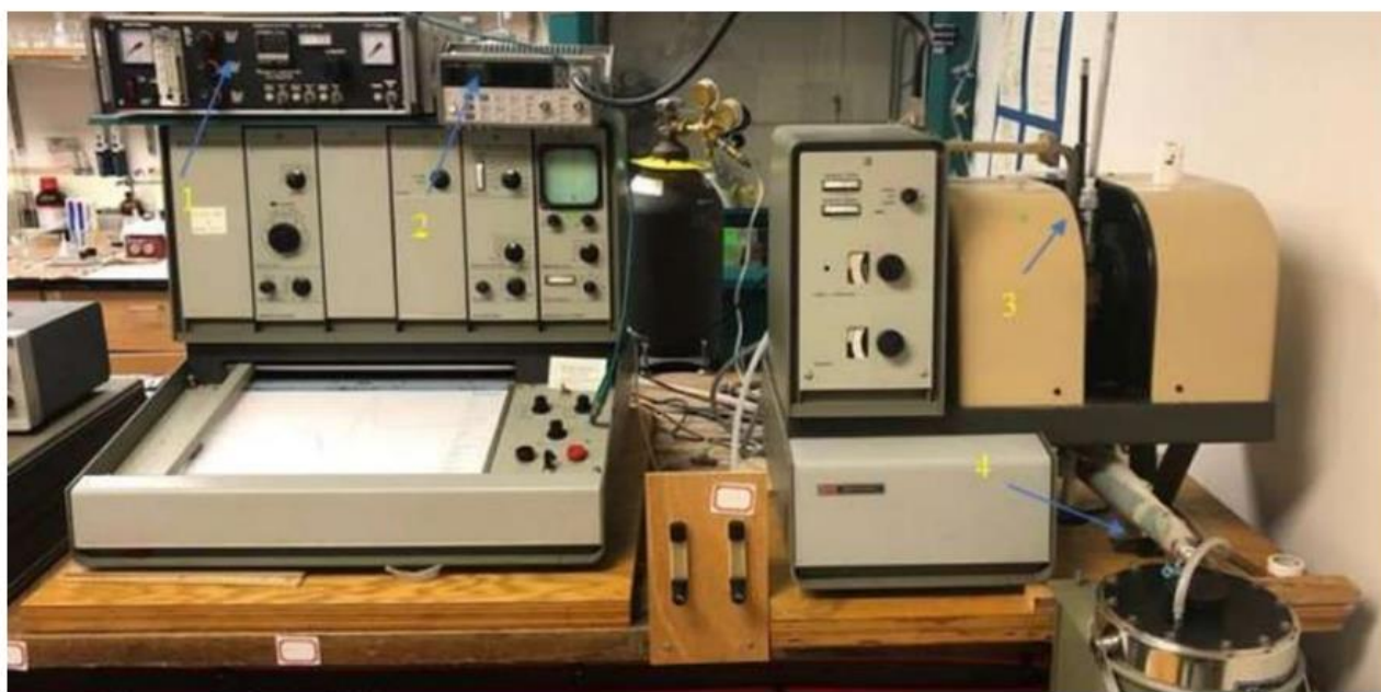
Figure 5 Instrument Setup Varian E-3 X-band Spectrometer. D.Petasis Lab, Allegheny College
