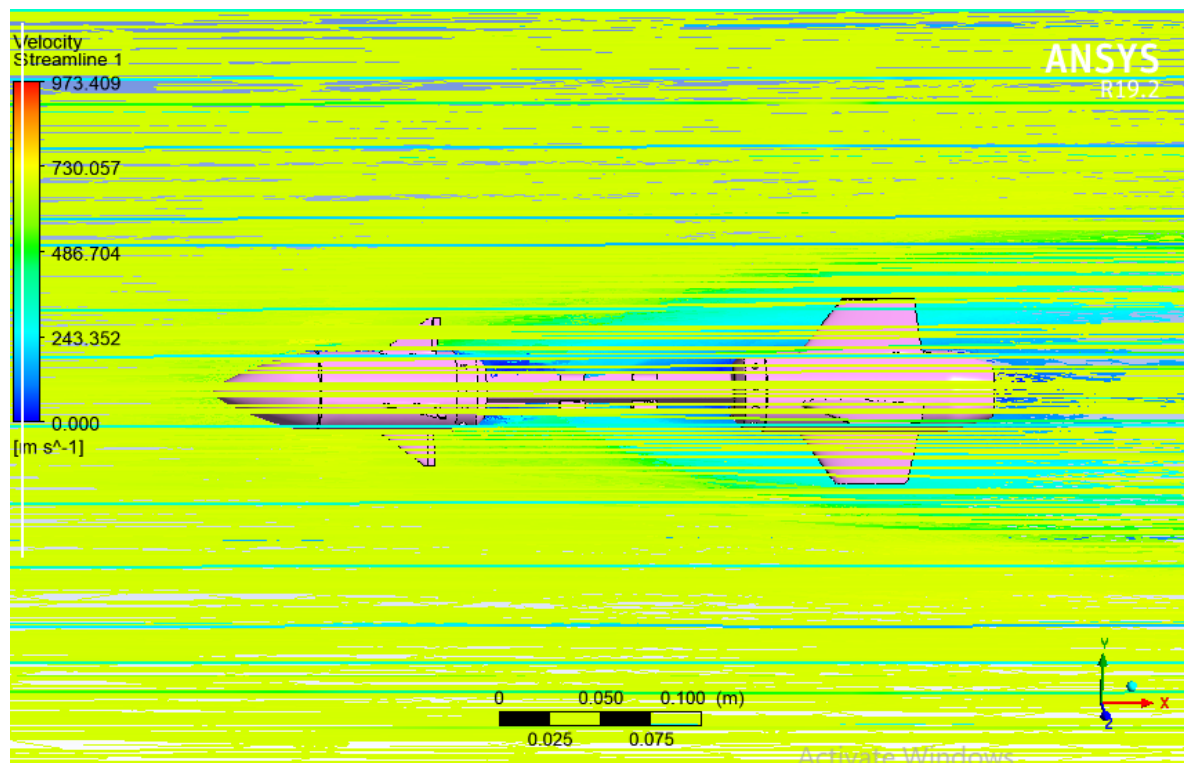
Fig: streamlines at 680 m/sec
