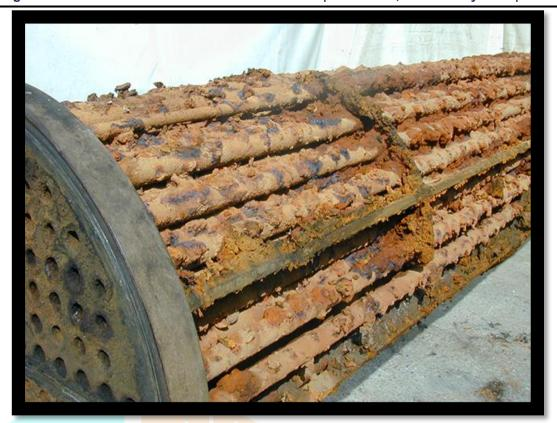
Fouling is a very dynamic and highly complex process, and it is governed by a wide range of interrelated parameters. These include the chemical composition and purity of the operating fluids, operating temperature of the heat exchanger, fluid flow rate, surface roughness or texture of the heat transfer surface, and the operating time. Changing any of these single parameters can accelerate or alter the mechanism of fouling, making it very difficult to predict and control.
