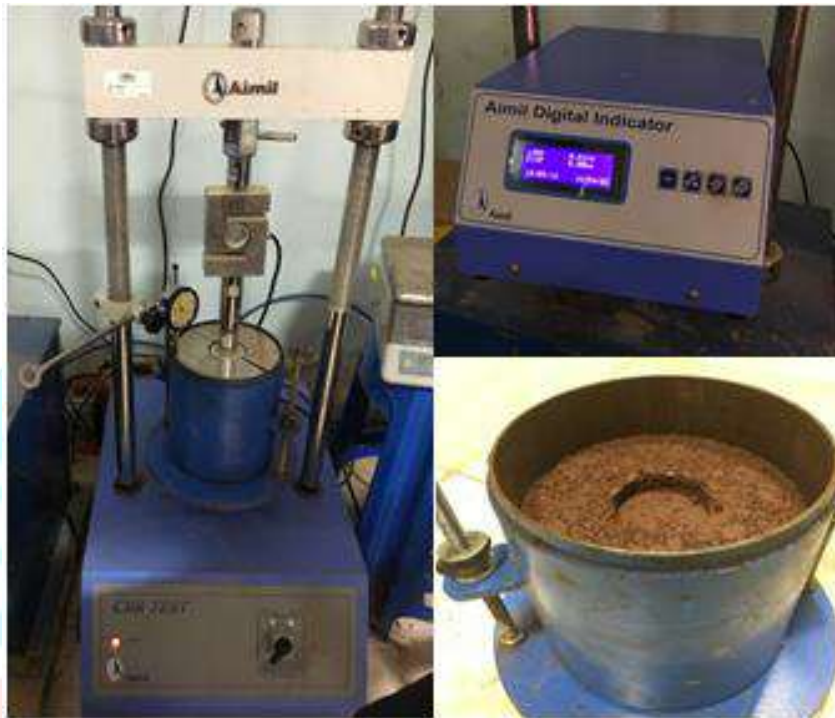
Figure 6.6 CBR setup and post test specimen
