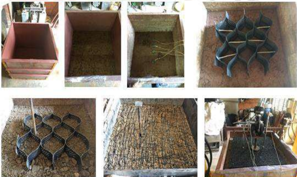
Figure 6.13 Various stages for the preparation of test section
