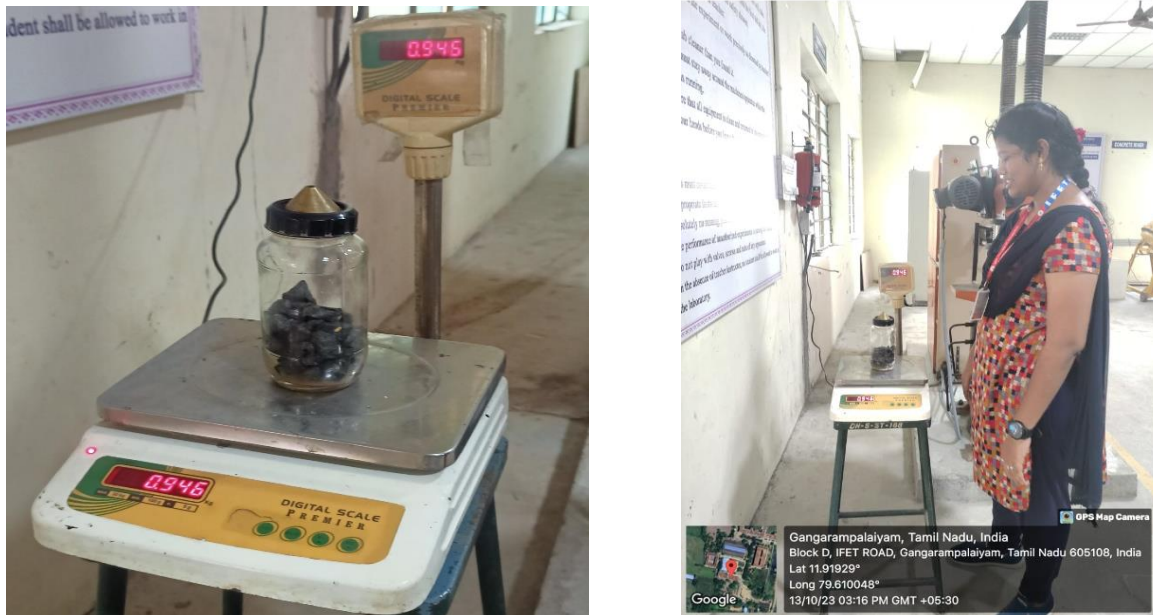
Fig 5.6 SPECIFIC GRAVITY OF COARSE AGGREGATE
