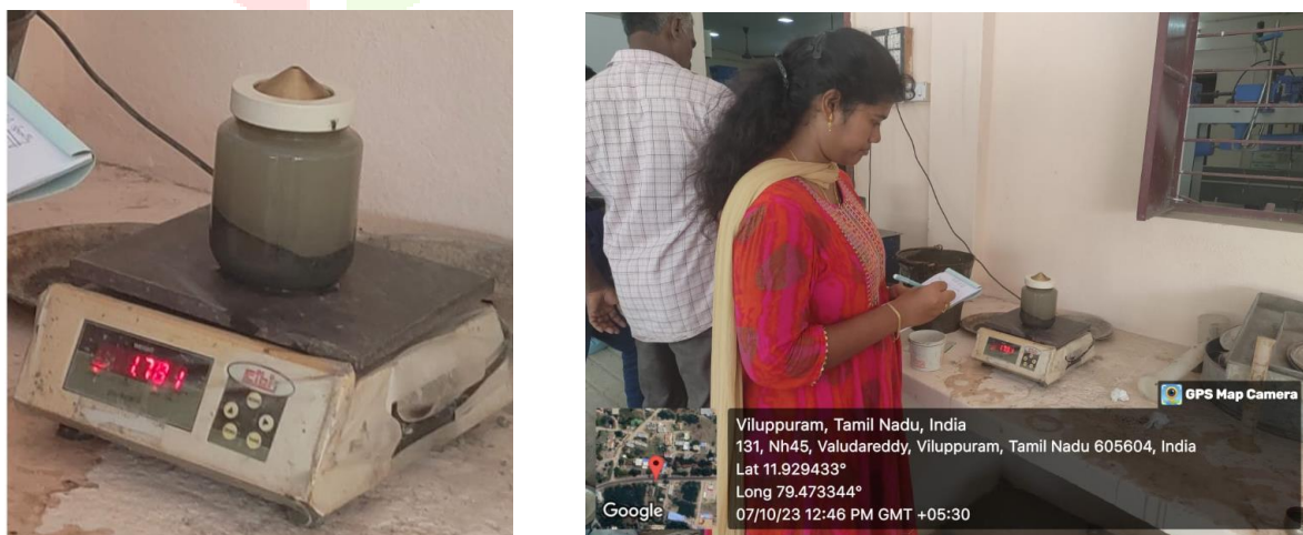
Fig 5.1 SPECIFIC GRAVITY OF CEMENT
