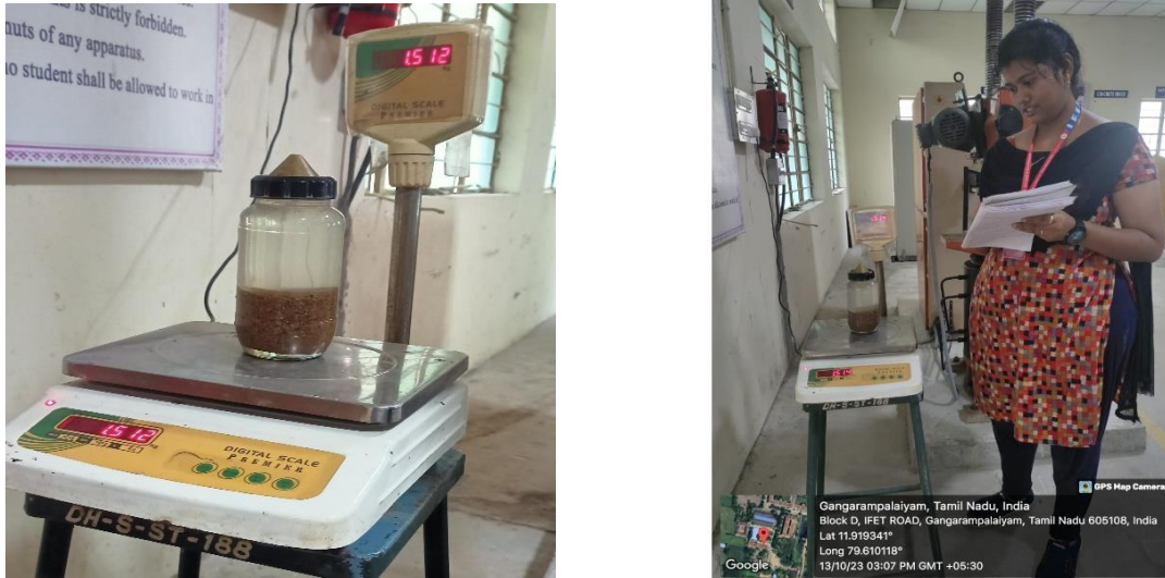
Fig 5.3 SPECIFIC GRAVITY OF FINE AGGREGATE
