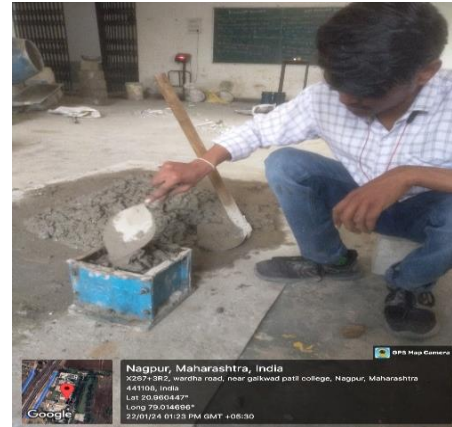
Figure 6.6 : Filing of concrete in molds
