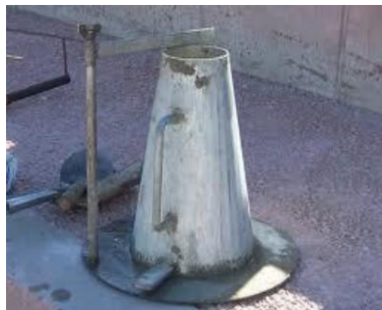
Figure 5.8 : Slump Testing Apparatus
