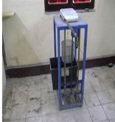
Figure 4.3 : Apparatus for specific gravity of coarse aggregate
