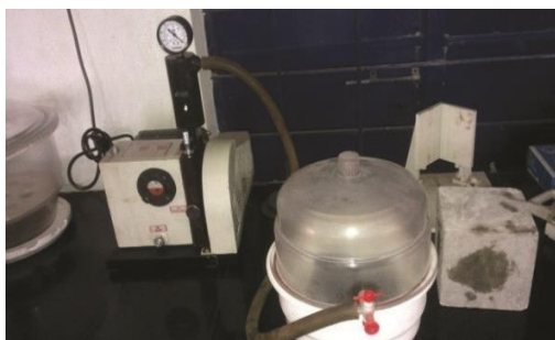
(c) Slices in vacuum chamber
