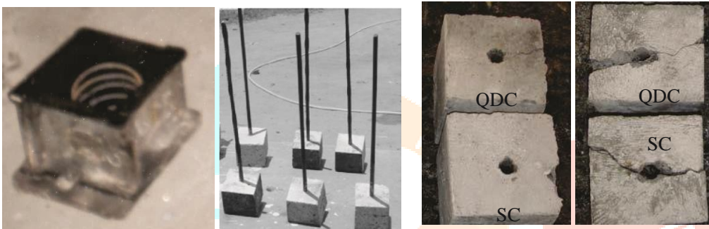
Spiral in the mould Specimen With plain bar With ribbed bar
