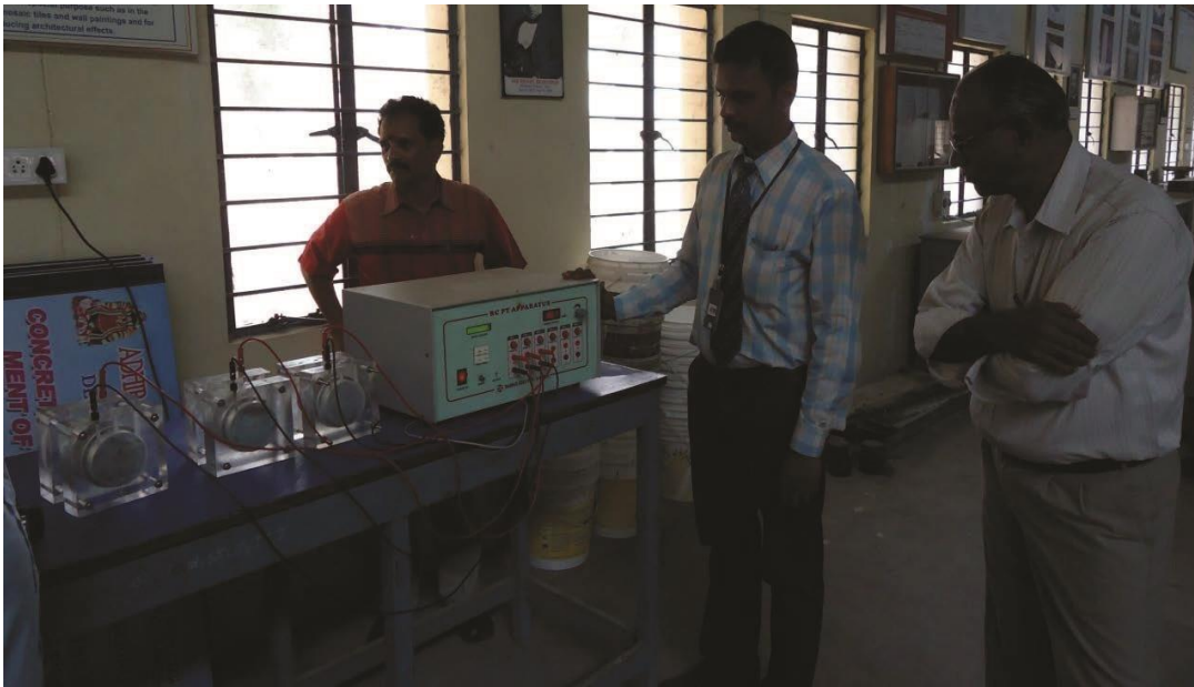
(e) RCPT in progress
