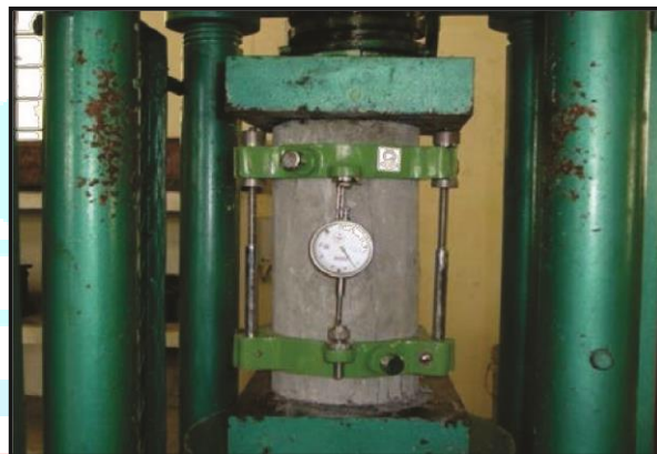
Fig. 4.5 Determination of Modulus of Elasticity of concrete
