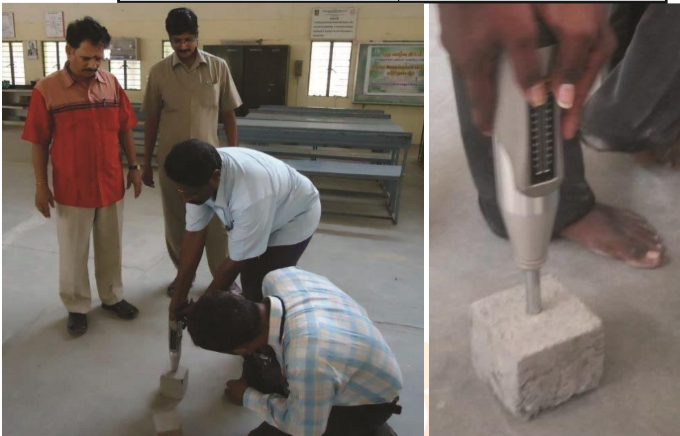
Fig. 4.8 Rebound Hammer Test in progress
