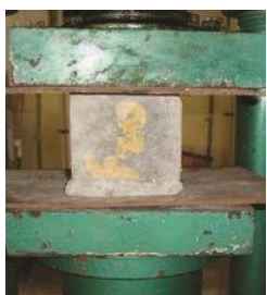
(a) Compression test
