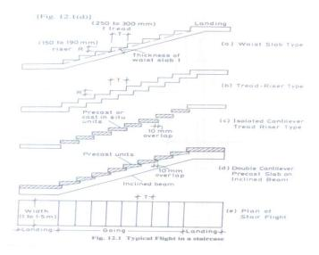
To break the monotony of climbing, the number of steps in a flight should not generally exceed 10 to 12.
