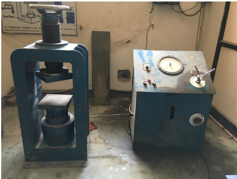
Fig. 3.18 Split Tensile Strength Test machine
