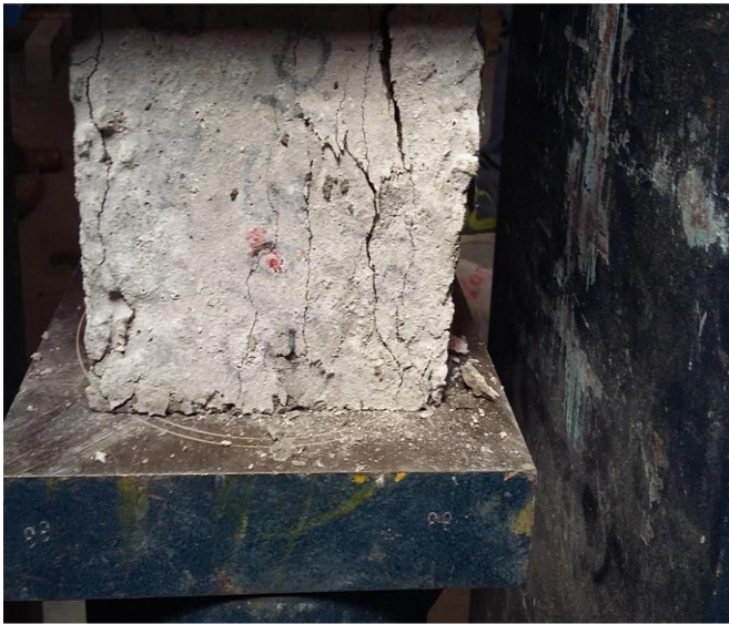
Fig. 3.17 Compressive Strength Testing
