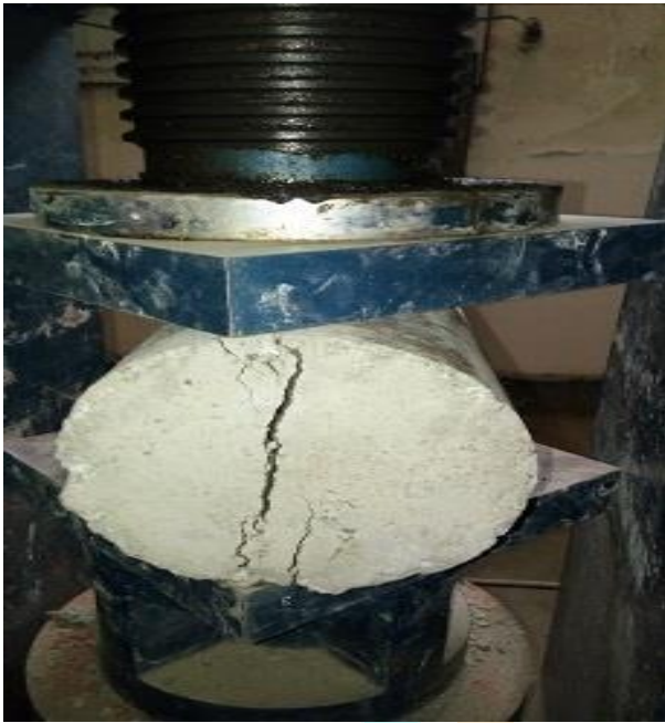
Fig. 3.19 Split Tensile Strength Testing of Cylinder
