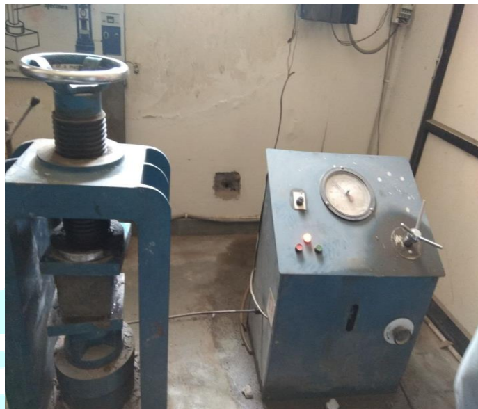
Fig. 3.16 Compressive Strength Testing Machine
