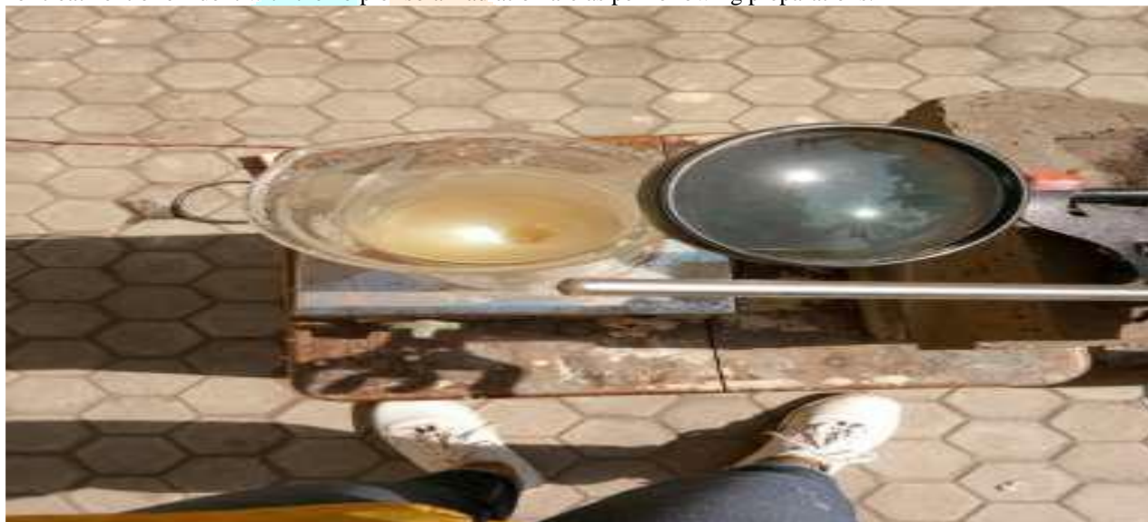
Figure 2: Solar Photo Fenton Reactor
