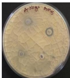
Fig.8. Inhibition zones for CuO nanoparticles against A. niger
