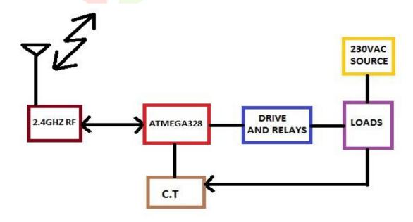
Figure 2. Functional block diagram of power measurement and controlled unit
