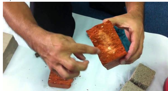
Fig 5: Water Absorption Test on Clay Bricks
