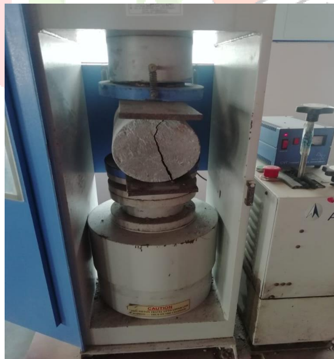
Fig 3.2: Split Tensile Strength Test
