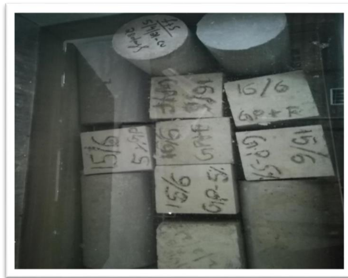
Fig 3.3 curing of cubes and cylinders
