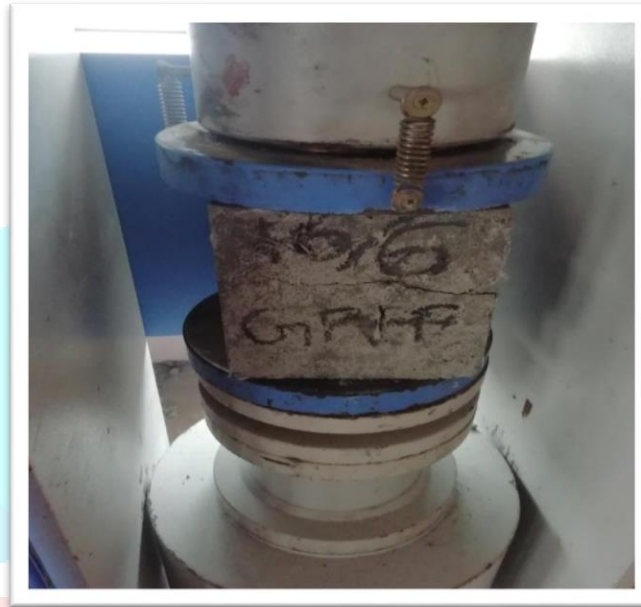
Fig 3.1: Compressive Strength Test
