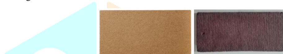
Fig.1 (a) Untreated soft board (b) PF resin-impregnated softboard
