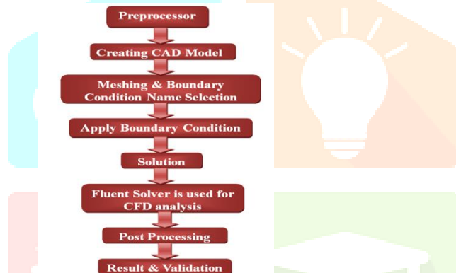
Figure:2 Algorithm used for Computational fluid dynamics analysis
