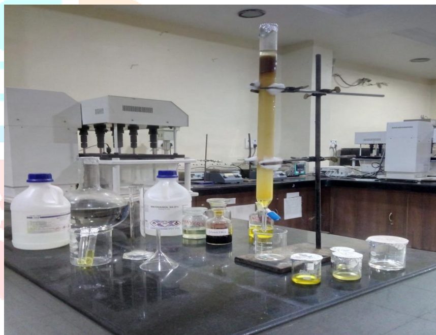
Figure. 5. Column Chromatography of methanol extract Of phyllanthus niruri
