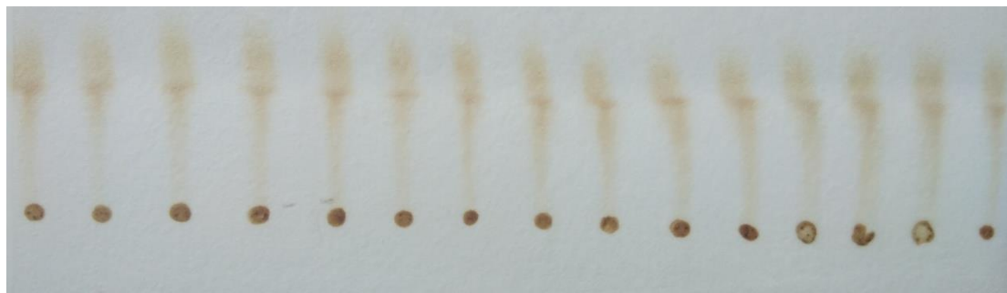
Figure. 7. Preparative Thin Layer Chromatography ethanol of phyllanthus niruri
