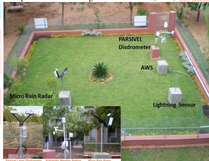
Fig.1: Photograph showing Atmospheric Laboratory at Yogi Vemana University, Kadapa. Ground-based PARSIVEL Disdrometer (PSD), AWS, Micro Rain Radar (MRR) and Lightning Sensor (LS). (Inset shows photograph of PSD, AWS, MRR and LS).
