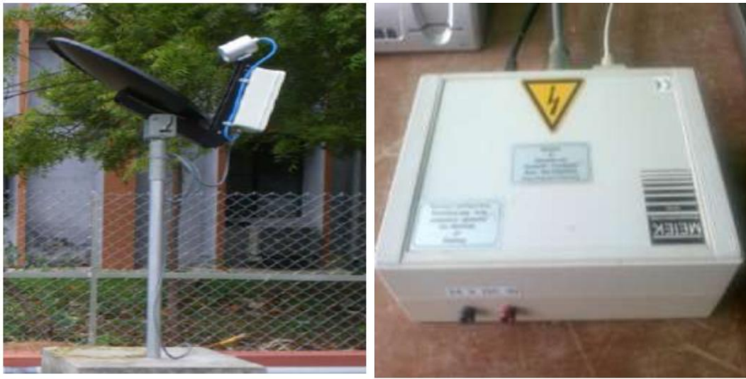
Fig.2: Experimental set-up showing (a) the Outdoor Unit and (b) indoor unit of the MRR
