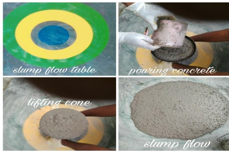
Fig. 3: Slump flow Process
