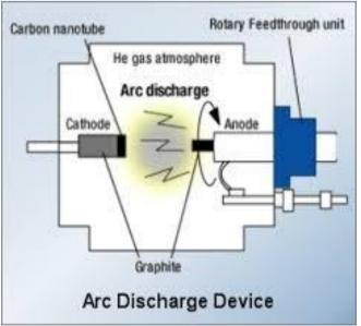
rods set finish to finish in an exceedingly location that's stuffed with depression and noble gas. The discharge evaporates the surface of 1 of the carbon electrodes, and creates a little rod-shaped deposit on the opposing conductor. the assembly of CNTs in high harvest depends on the uniformity of the plasma arc, and therefore the temperature of the deposit growing on the carbon conductor. 30-38
