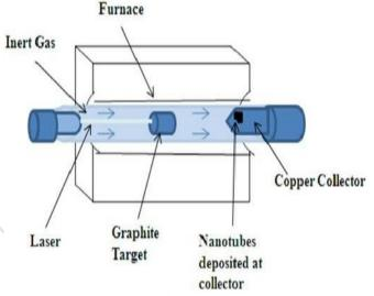
heat treatment in an exceedingly vacuum at one thousand °C to eradicate the C60 and different fullerenes. the primary optical maser vaporization pulse was trailed by a succeeding pulse, to vaporize the target additional systematically<sup>30-38</sup>.
