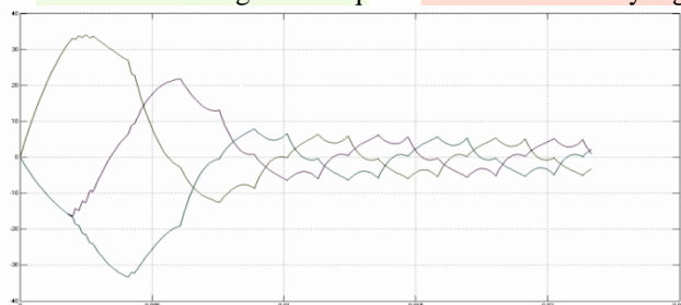
Fig. 17 Scope view of 3 phase current of PMSM with fuzzy logic controller
