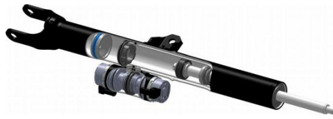
Figure 2: Valve-actuated Suspension system
