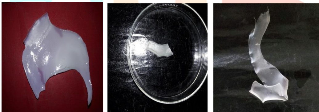
Plate 4. Preparation of CMC bioplastic treated with acetone
