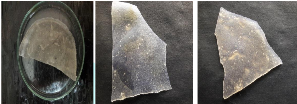
Plate 3. Preparation of corn starch bioplastic treated with acetone
