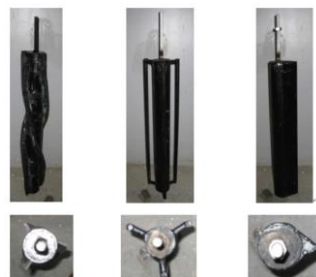
Three disturbing flow devices of anchor cables: Spiral fringe, Control rod and Fairing
