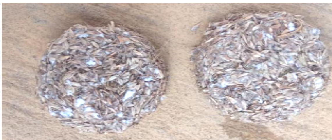
Fig 2: Briquette Made By Rice Husk
