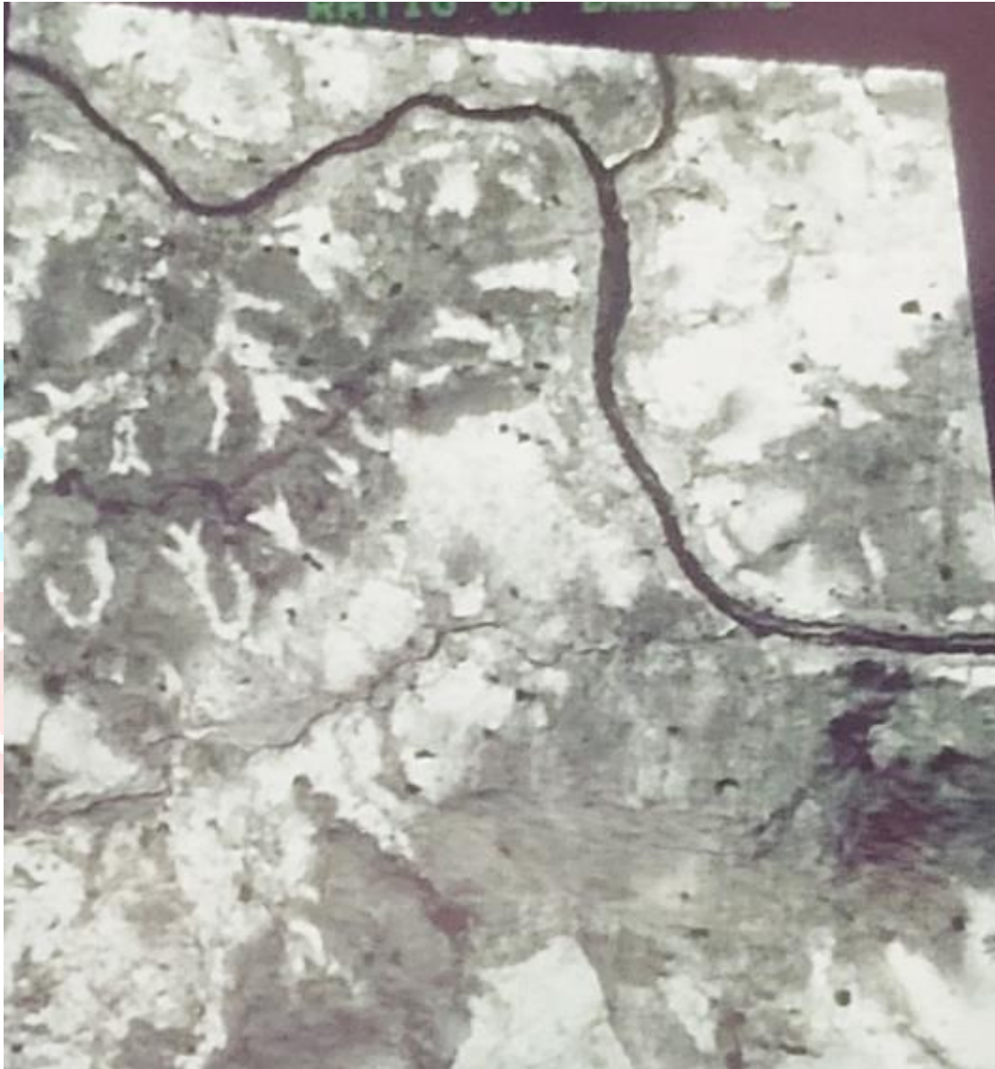
Fig.8 Paleo-drainage through Band ratio 4/2 along village; Sonadih
