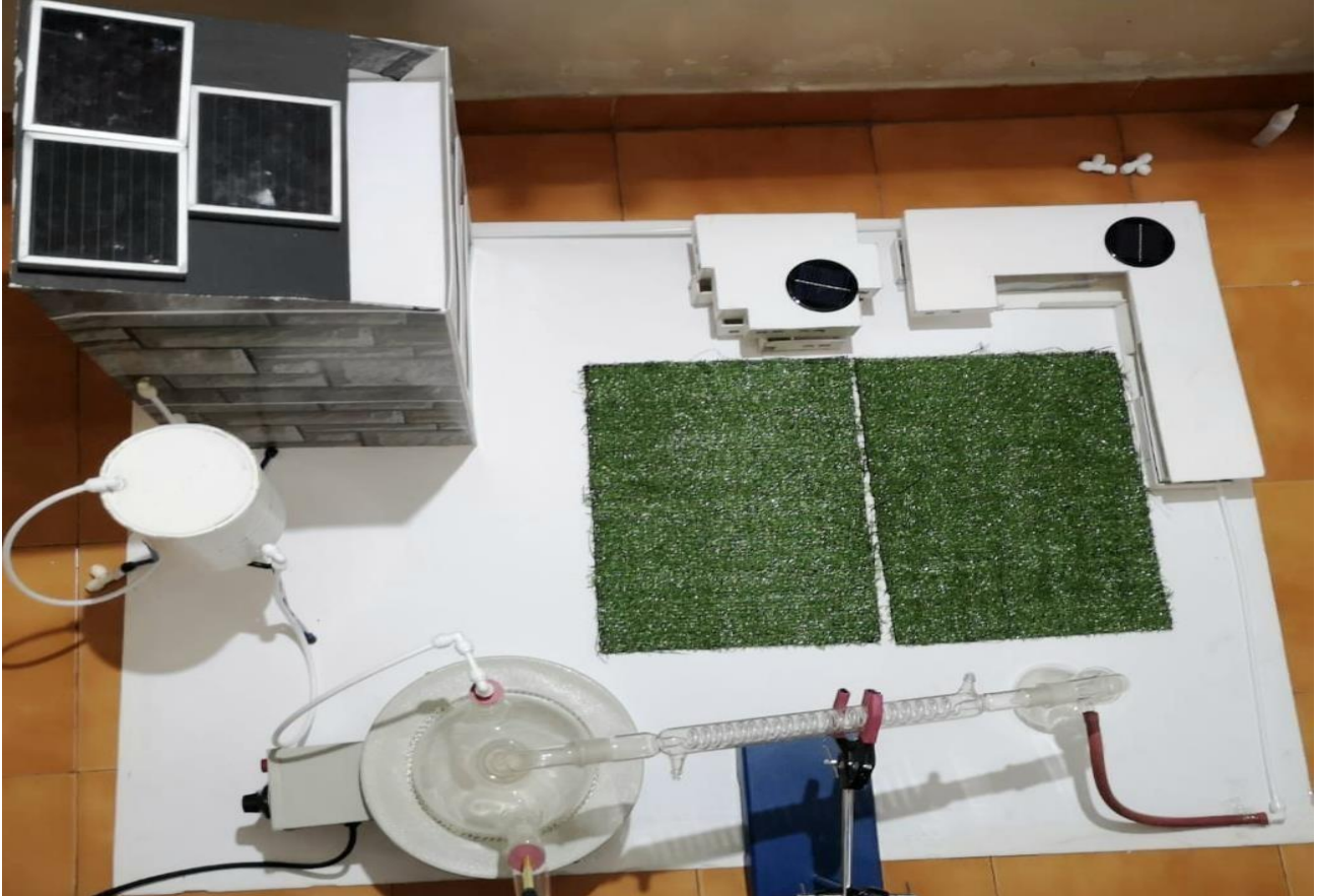
Fig: -2overview of solar distillation process 1
