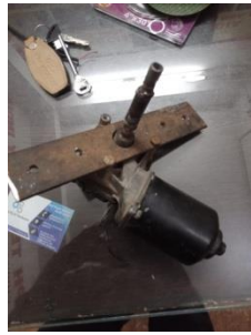
Figure: DC motor (bevel geared with speed reduction high torque motor)
