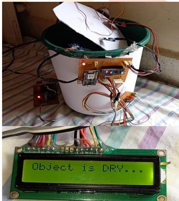
Fig. 11. Detection of dry waste
