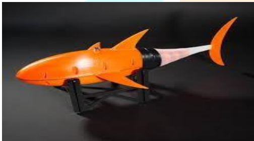
Fig 6: The Solid works designed 3D prototype of the Robot Fish
