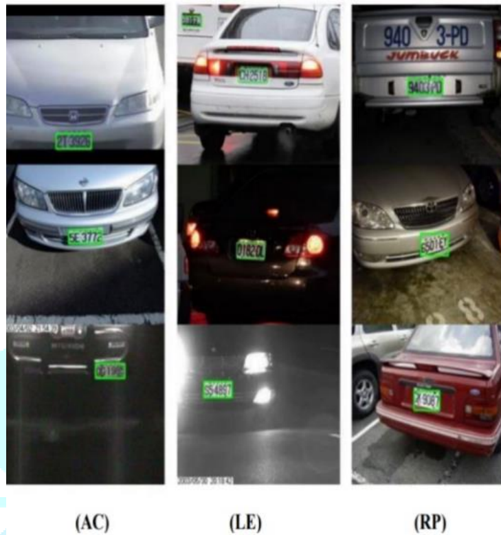
Figure 3. Detection results of lps detected by our method. Pointed detection of lps showing the robustness of algorithm even have different camera distance, illumination, angle, and several ambiguities.
