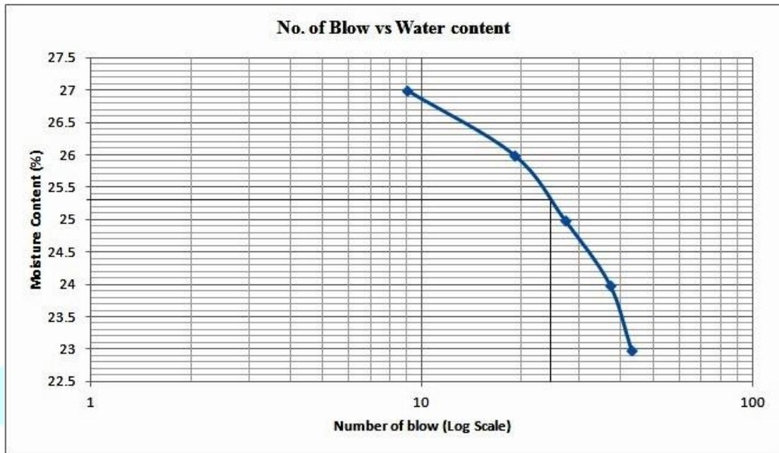
Fig 6.1 - Liquid limit curve
