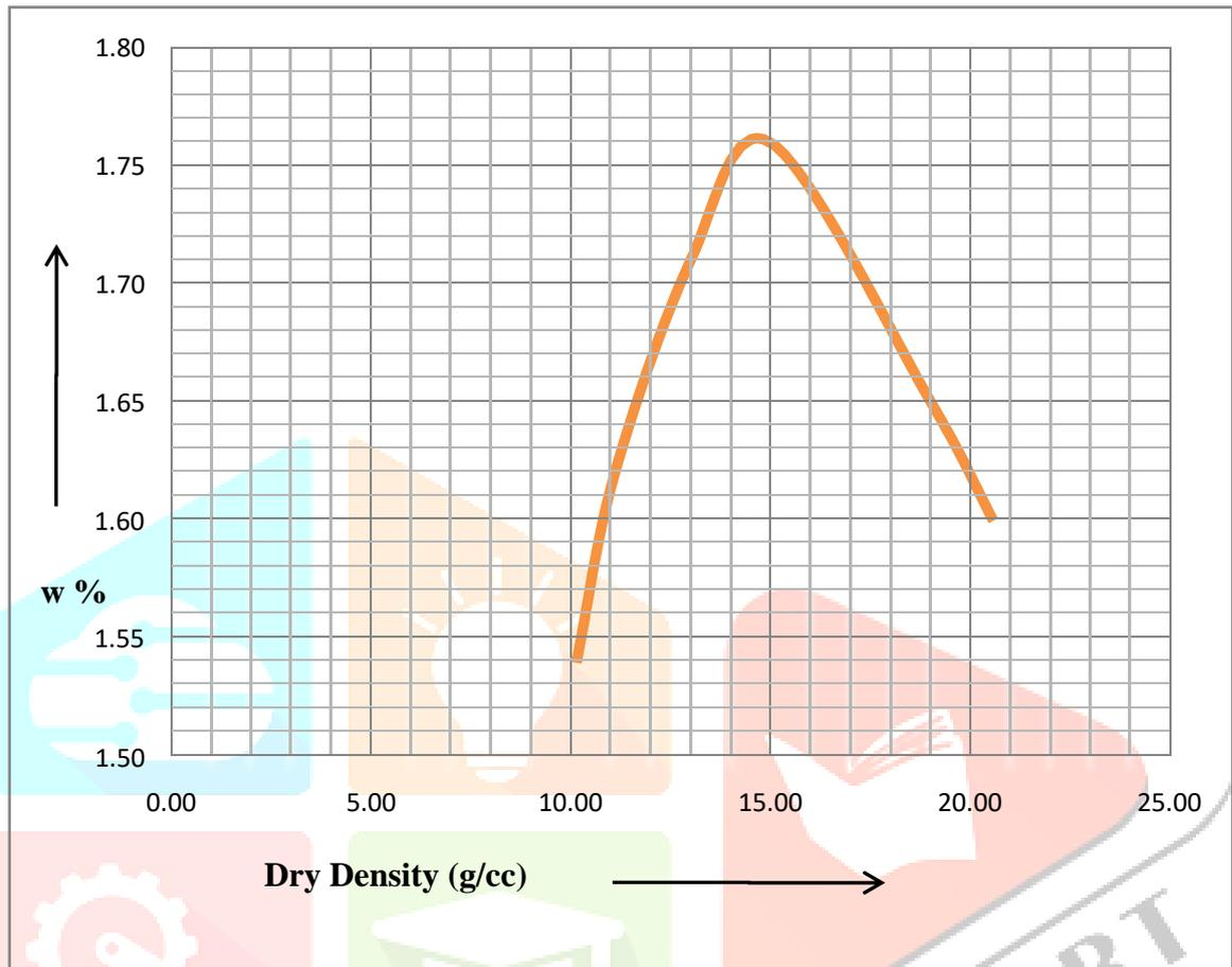
**Fig 6.3 - Curve between water content and Dry density**
