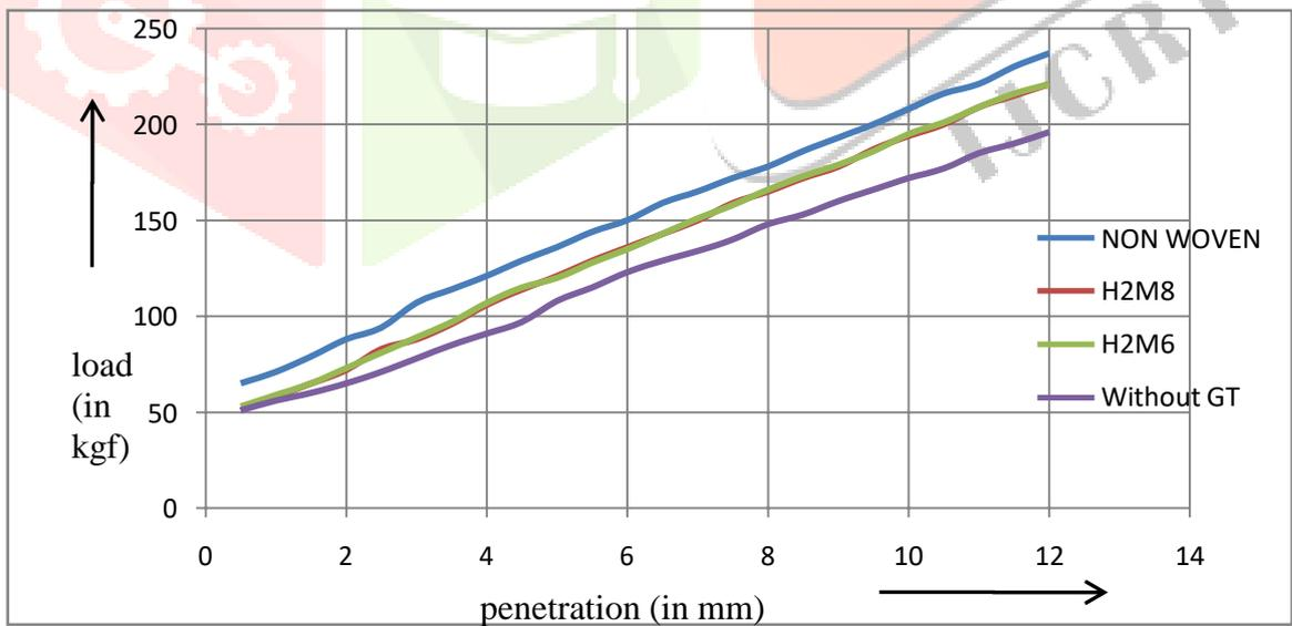
**Figure 8.2 Load-penetration curves with synthetic fibre (0.5%) and coir geotextiles placed at H/3 from top**
