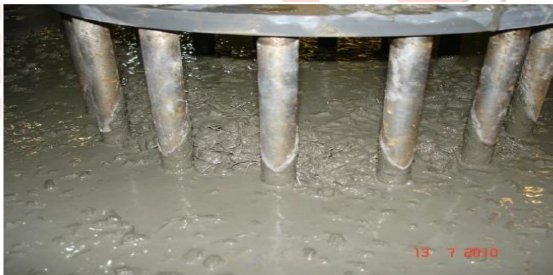
Figure 3.10: Fibres and large aggregates are nested around the steel rods in an earlier trial version of Mix 6 that had met the flow-ability criterion
