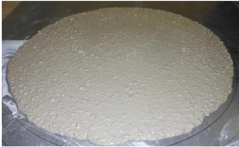
Figure 3.4: Horizontal spread of SCC Mix 3
