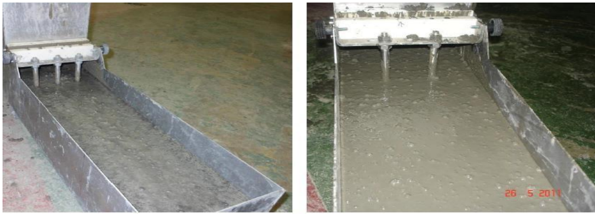
Figure 3.14: Flow and passing ability of SCC Mix 5 (left) and Mix 6 (right)
