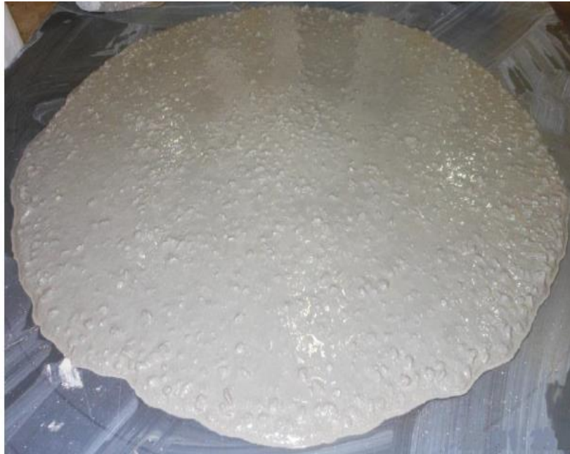
Figure 3.2: Horizontal spread of SCC Mix 1
