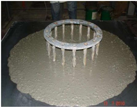
Figure 3.8: Flow and passing ability of SCC Mix 4
