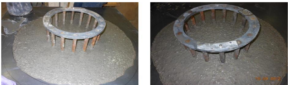
Figure 3.7: Flow and passing ability of SCC Mix 2 (left) and Mix 3 (right)
