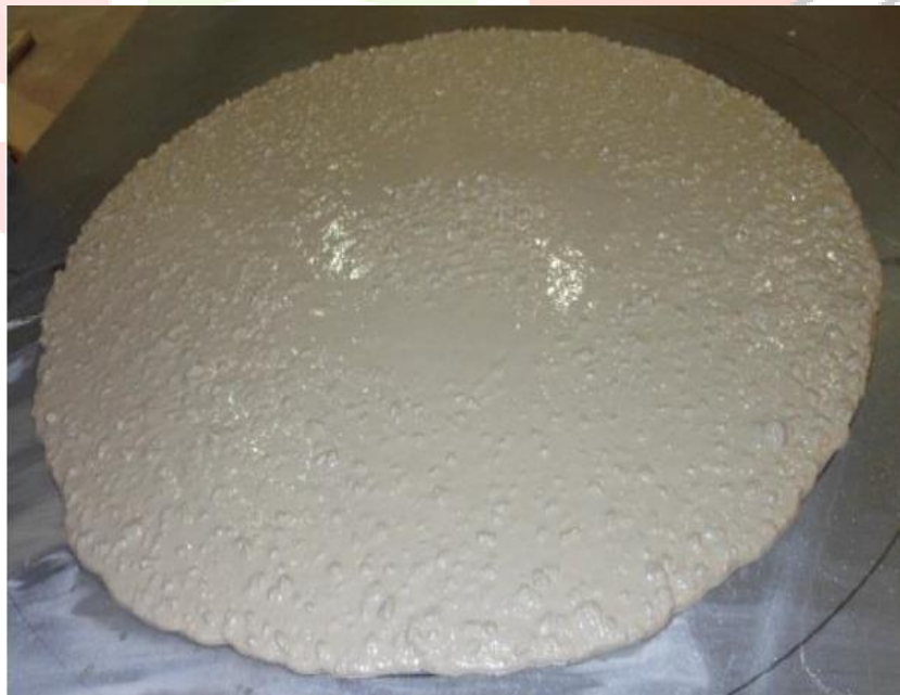
Figure 3.3: Horizontal spread of SCC Mix 2
