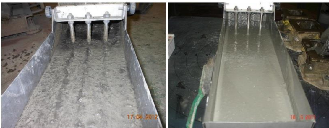
Figure 3.13: Flow and passing ability of SCC Mix 3 (left) and Mix 4 (right)
