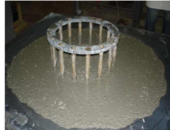
Figure 3.9: Flow and passing ability of Mix 5 (left) and Mix 6 (right)
