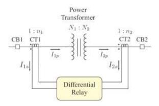
According to Fig. 2, under normal operation conditions, the CT secondary currents I1s and I2s are approximately equal. However, when an internal fault occur, this condition is no longer verified, and the difference between I1s and I2s becomes much large.
