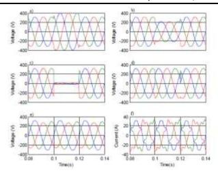
Most encountered power system problems. a) Voltage swells. b) Voltage sags. c) Voltage interruption. d) Frequency variation. e) Voltage unbalance. f) Harmonics.
