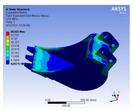
Fig.12: Equivalent Stresses of Excavator Bucket
