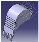
Fig.5: CAD model of Bucket
