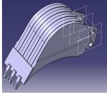
Fig. 3: CAD model of Bucket
