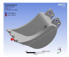
Fig.9: Forces Applied on Excavator Bucket
