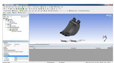
Fig. 8: Meshed View of Existing Excavator Bucket
