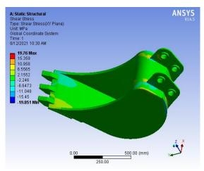
Fig.11: Shear Stress due to loading on Excavator Bucket
