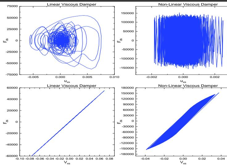
Figure 3 when aspect ratio 1.0, Damper force-displacement and velocity loops for PVD damper located at stiff edge and flexible edge under Imperial Valley, 1940 Earthquake
