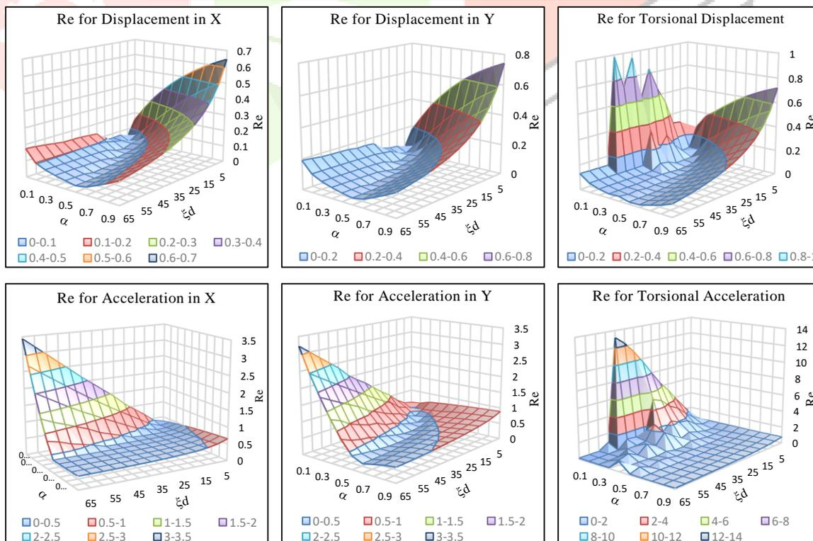
Figure 4 When aspect ratio 1.2, Effect of exponent ( $\alpha$ ) and damping ratio ( $\xi_d$ ) on response ratio,  $R_e$  for PVD various displacement and acceleration under Imperial Valley, 1940 Earthquake
