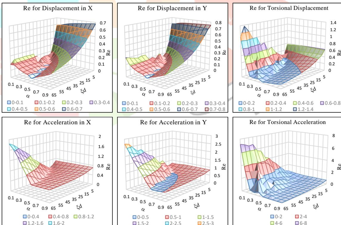
Figure 7 When aspect ratio 1.2, Effect of exponent ( $\alpha$ ) and damping ratio ( $\xi d$ ) on response ratio. Re for PVD various displacement and acceleration under Kobe, 1995 Earthquake
