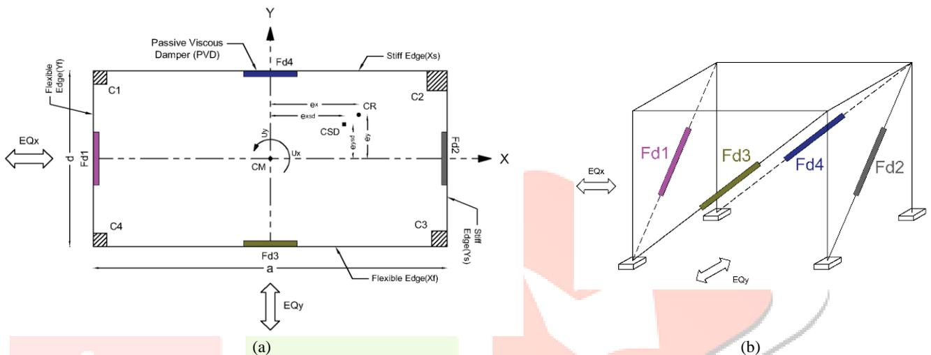
Figure 1 (a) Plan of two-way asymmetric system (b) Isometric view of system showing arrangement of dampers for structure installed with PVD
