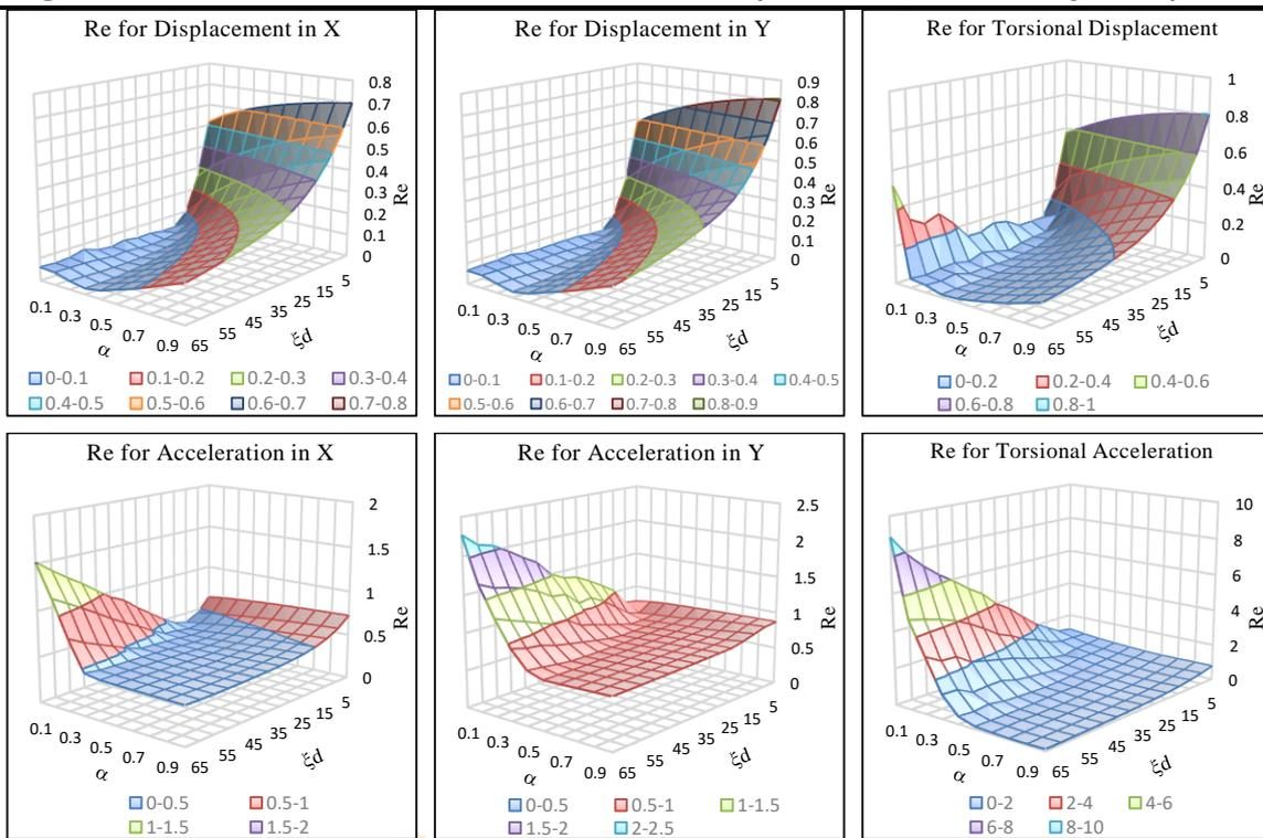
Figure 8 When aspect ratio 1.2, Effect of exponent ( $\alpha$ ) and damping ratio ( $\xi d$ ) on response ratio. Re for PVD various displacement and acceleration under Bhuj, 2001 Earthquake
