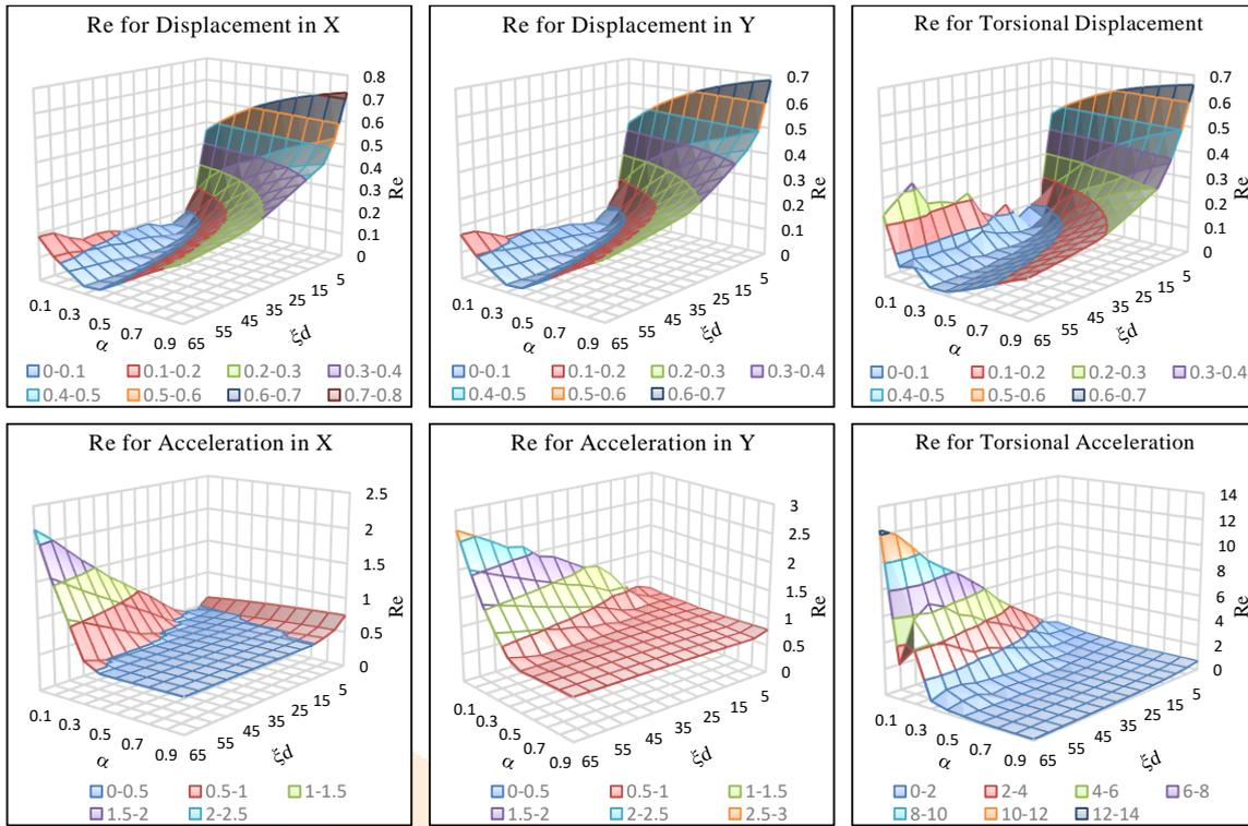
Figure 6 When aspect ratio 1.2, Effect of exponent ( $\alpha$ ) and damping ratio ( $\xi d$ ) on response ratio. Re for PVD various displacement and acceleration under Northridge, 1994 Earthquake
