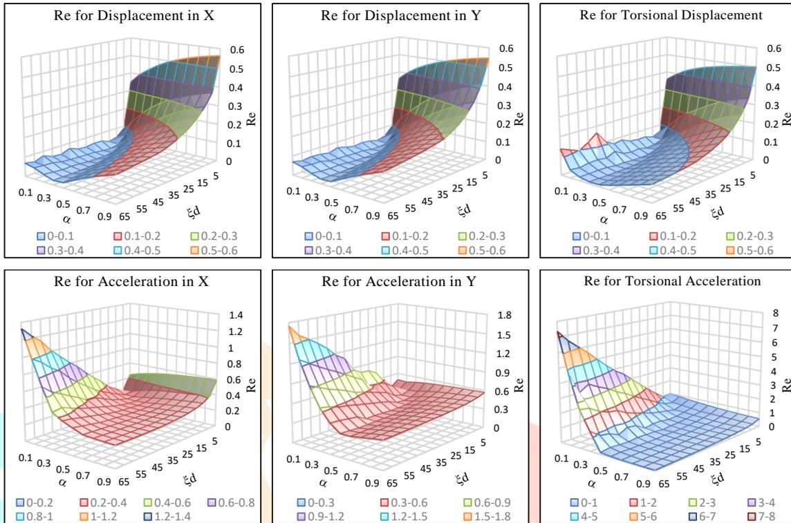
Figure 5 When aspect ratio 1.2, Effect of exponent ( $\alpha$ ) and damping ratio ( $\xi_d$ ) on response ratio.  $R_e$  for PVD various displacement and acceleration under Loma Prieta, 1989 Earthquake
