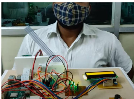
Fig: 7.3 Temperature normal, Mask detection and gate will be open
