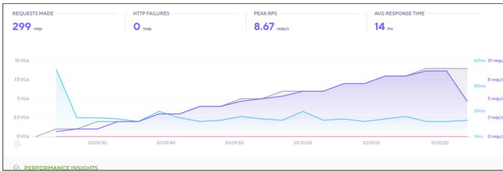
Fig:4: the above image shows the representation of the change in the load that happened while testing with 10 users. The image shows peak RPS, AVG response time, and failures.
