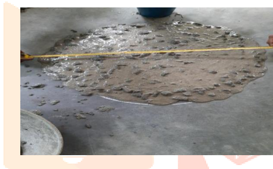
Fig. 2.1 Slump Flow Test
