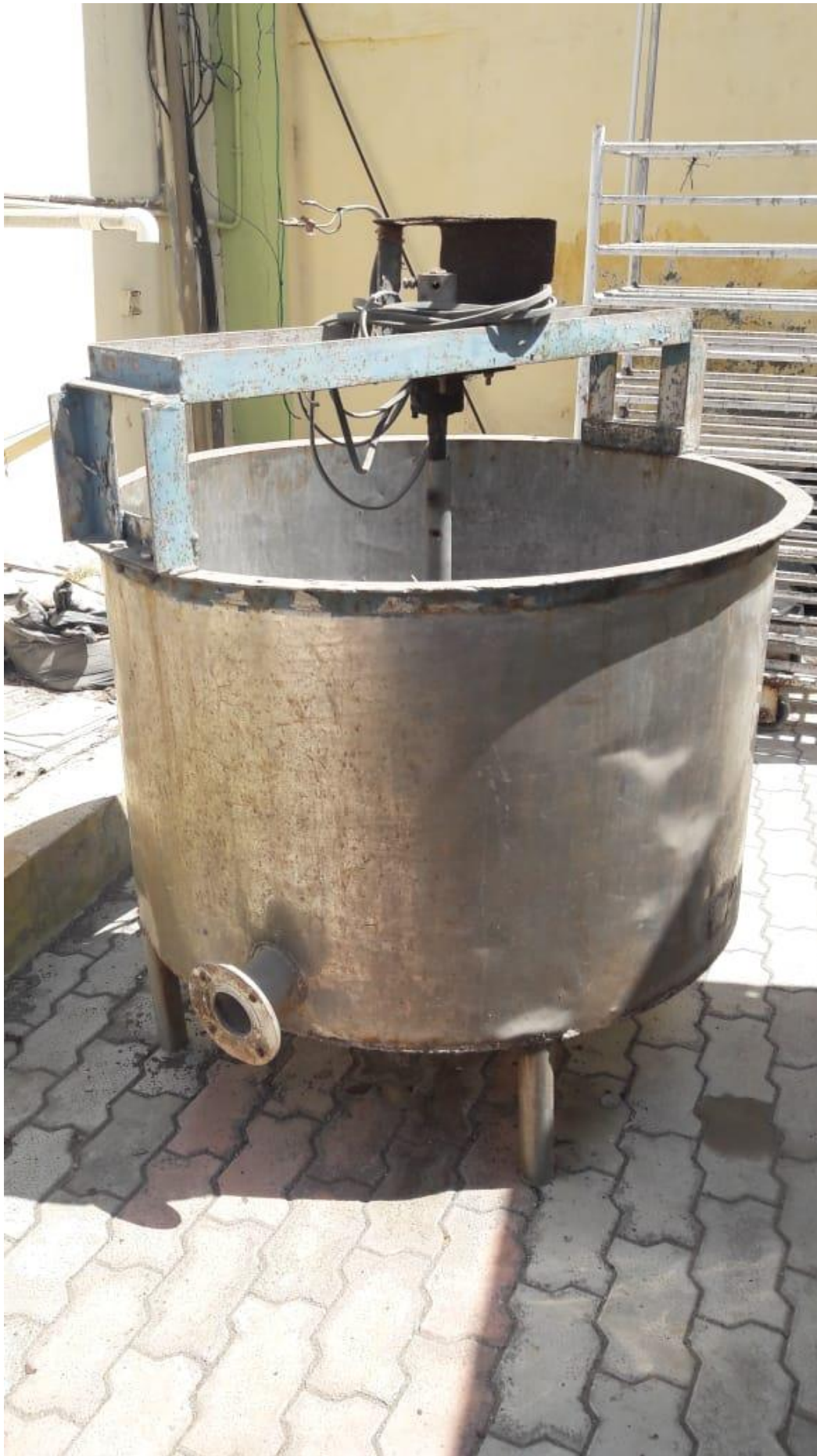
Fig:4CHEMICAL CONVERSION OF CRAB HARD SHELL TO SOFT SHELL BY BLENDING WITH HYDROCHLORIC ACID IN BLENDER
