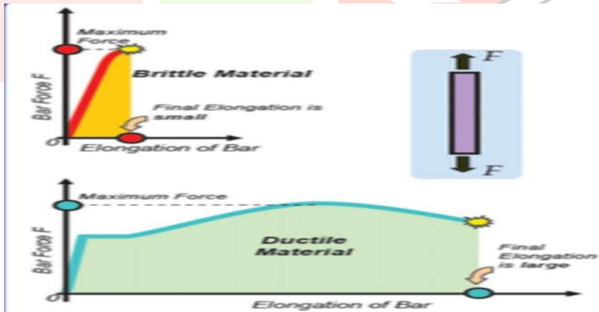
Figure 7: Tension test on materials ductile versus brittle materials
