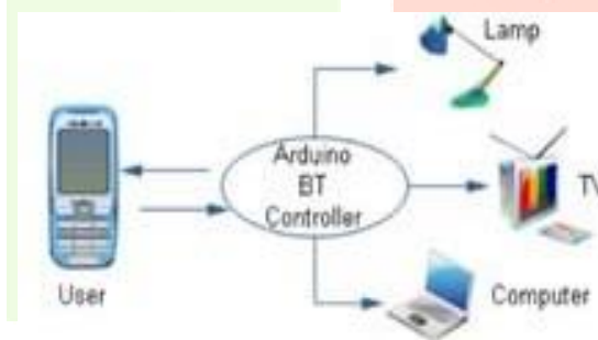
Fig: Block diagram of Home automation system
