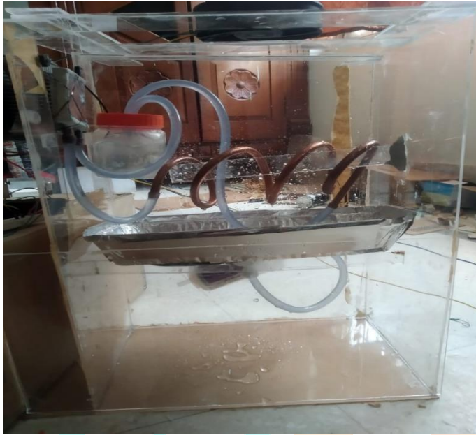
Fig.5: AWG system and water level control module
